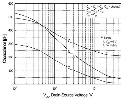
**Figure 5. Capacitance Characteristics**
