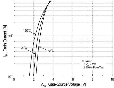
**Figure 2. Transfer Characteristics**
