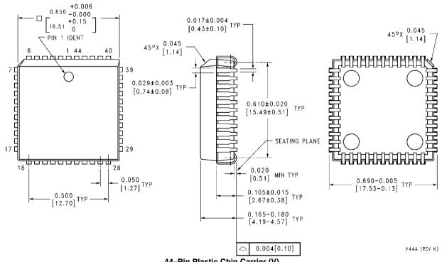
44-Pin Plastic Chip Carrier (V)
