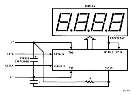
FIGURE 7. Four Wire Remote Display
