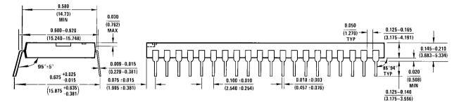
40-Pin Molded Dual-In-Line Package (N) Order Number MM5452N or MM5453N NS Package Number N40A N40A (REV E)
