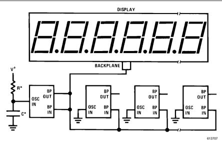
\*The minimum recommended value for R for the oscillator input is  $9 \text{ k}\Omega$ . An RC time constant of approximately  $4.91 \times 10^{-4}$  should produce a backplane frequency between 30 Hz and 150 Hz.
