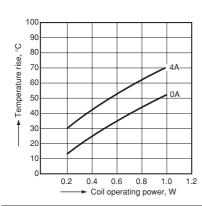
4.-(2) Coil temperature rise Tested Sample: S4EB-24V, 4 Form A
