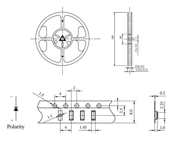
Reel Lead Min.60mm No LEDs
