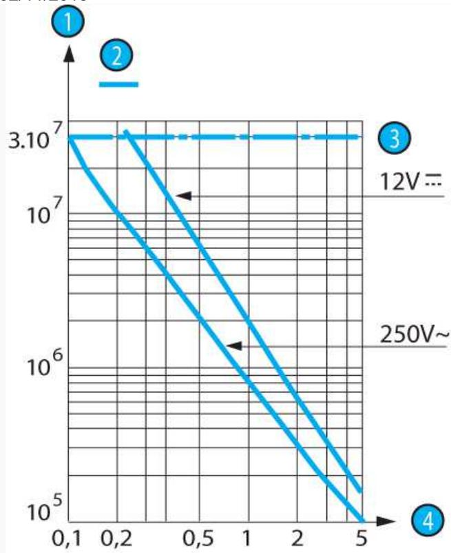
Models 83 170 8 and 83 170 9 are designed to operate equally well on dual-current (1 mA 4 V minimum) or medium-current (5 A maximum) circuits. However, a given product should only be used to switch one type of circuit during its working life.
