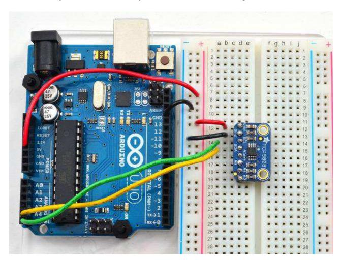
• Connect Vdd to the power supply, 3V or 5V is fine. Use the same voltage that the
