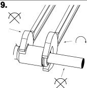
Tighten nipple. (torque 11 Nm)
