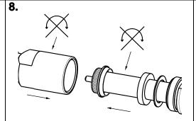
Push prepared cable into connector body.
