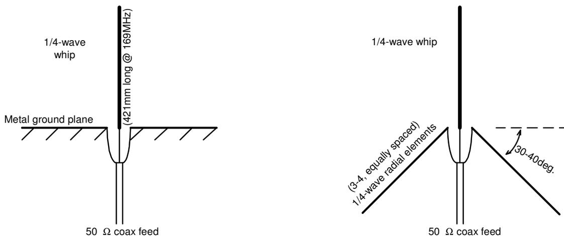
Fig.8: Quarter wave antenna / ground plane configurations
