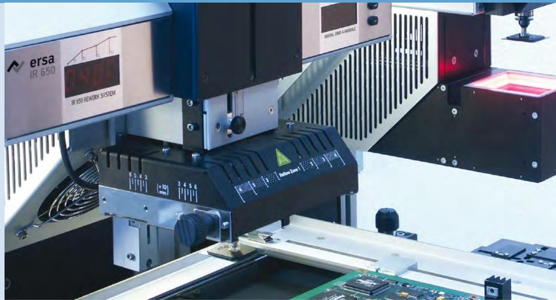
The IR/PL 650 provides a very high heating power (4,400 W) for large and complex PCBs. Offering a high degree of automation, the IR/PL 650 requires only little user intervention. This guarantees stable and repeatable rework processes for all applications.
