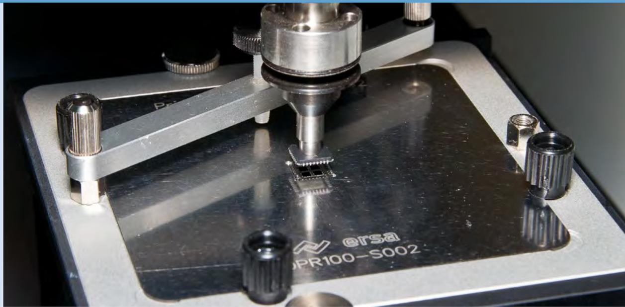
The Erska DIP&PRINT STATION enables the user of an Erska rework system to easily, reliably and reproducibly perform the preparatory work on the component (application of solder paste or flux).
