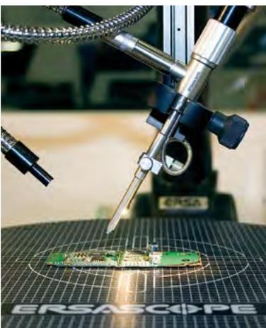
*High magnification and viewing angles from 0 to 90° offer maximum inspection flexibility*
