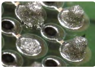
BGA – paste print: insufficient solder
