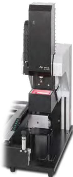
The PL 650 module is the second generation precision placement system designed for the largest range of components. It provides increased automation and excellent repeatability. A highly sophisticated and fully automated, pressure triggered component placement head drops off the component at the same contact pressure (1.5 N) as an in-line pick & place machine.
