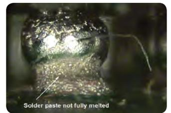
PBGA – scaling: insufficient heat
