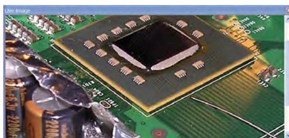
Rework process visualization with live image window
