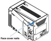
3, Join the nails on the back of the display module with the inset part of the main module, and push it in.
