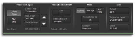
Spectrum analyzer style controls simplify waveform analysis in the frequency domain.
