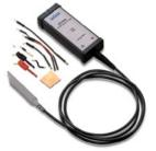
The ZS Series probes provide high impedance and an extensive set of probe tips and ground accessories to handle a wide range of probing scenarios. The high 1 M $\Omega$  input resistance and low 0.9 pF input capacitance mean this probe is ideal for all frequencies. The ZS Series probes provide full system bandwidth for all Teledyne LeCroy oscilloscopes having bandwidths of 1 GHz and lower.
