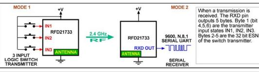
The RFD21733 stays in (2 uA) deep sleep, until any combination of the 3 buttons are pressed, then it will transmit the state of all 3 inputs. With every transmission it also sends it's unique 32 BIT ESN (Electronic Serial Number).
