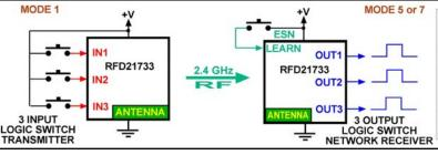
OUT1, OUT2 or OUT3 (follow) output any transmission received by the transmitter switch states IN1, IN2 or IN3. Depending on the configured mode there is a 20 or 500 millisecond hang time. The receiver will only respond to transmitters if it has learned their ESNs.
