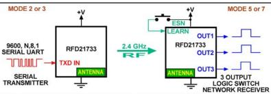
When a byte is received by the serial transmitter, OUT1, OUT2, OUT3, follow the states in bit position 4,5,6. Depending on the configured mode there is a 20 or 500 millisecond hang time. The receiver will only respond to transmitters if it has learned their ESNs.
