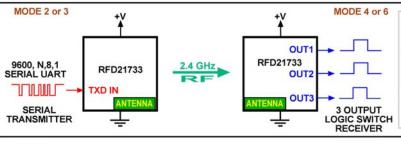
When a byte is received by the serial transmitter, OUT1, OUT2, OUT3, follow the states in bit position 4,5,6. Depending on the configured mode there is a 20 or 500 millisecond hang time.
