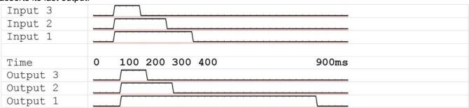
The second diagram shows the same operation at the transmitter, but with the receiver configured with a 20ms hang time.
