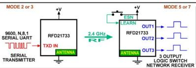
When 5 bytes are received in a row from a serial transmitter, OUT1, OUT2, OUT3, follow the states in Byte1, bit position 4,5,6. Depending on the configured mode there is a 20 or 500 millisecond hang time. The receiver will only respond if byte 2-5 contains it's ESN.
