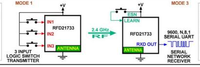
When a transmission is received. The RXD pin outputs 5 bytes. Byte 1 (bit 4,5,6) are the transmitter input states IN1, IN2, IN3. Bytes 2-5 are the 32 bit ESN of the switch transmitter. The receiver will only respond to transmitters if it has learned their ESNs.
