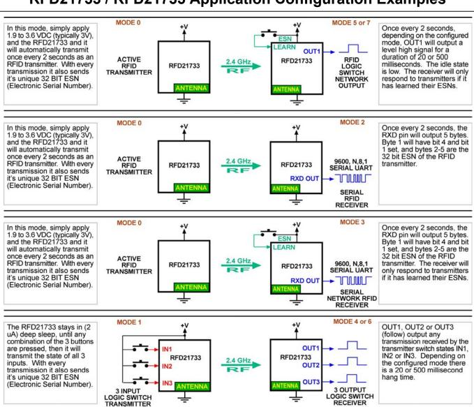
The RFD21733 stays in (2 uA) deep sleep, until any combination of the 3 buttons are pressed, then it will transmit the state of all 3 inputs. With every transmission it also sends it's unique 32 BIT ESN (Electronic Serial Number).
