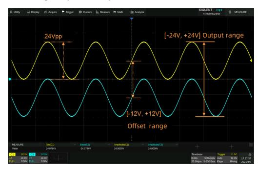
24Vpp analog output superimposed with  $\pm$  12 Vdc offset, providing a maximum output range of  $\pm$  24 V (48 V).
