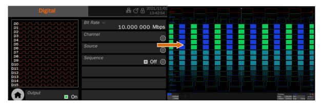
Purchase the corresponding digital bus kit to get 16-channel LVTTL or LVDS output with a bit rate of 1  $\mu$ bps ~ 1 Gbps. Combine the digital bus with the analog channels to realize mixed-signal outputs.
