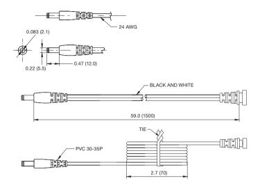
Wire type: VW-1 80°C 300V L=1500 mm 2468 20 AWG for 5 V output, 22 AWG for 9 V ouput, 24 AWG for 12 V output, 2C Black and White. Black - Negative, White - Positive
