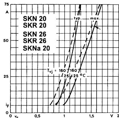
Fig. 6 Forward characteristics
