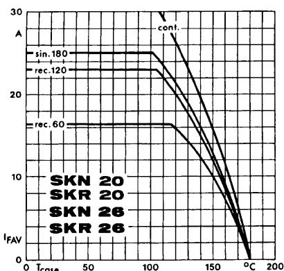
Fig. 3a Rated forward current vs. case temperature
