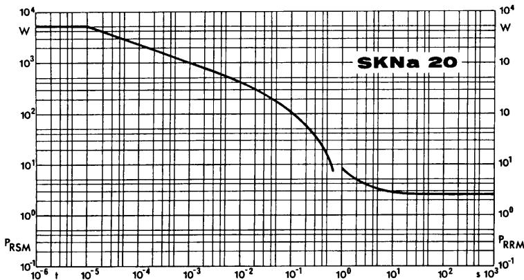
Fig. 11 Rated reverse power dissipation vs. time
