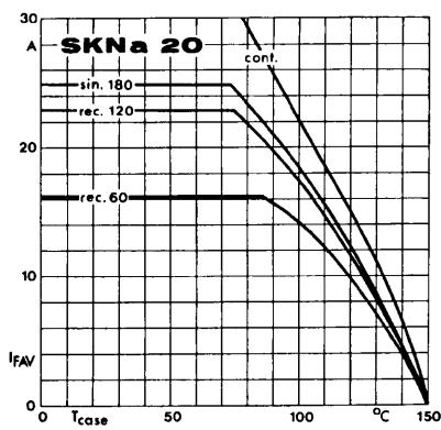
Fig. 3 b Rated forward current vs. case temperature
