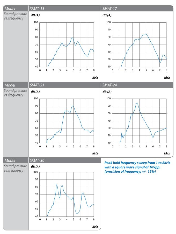
All measurements are made @ 30 cm in free air @ 21°C.
